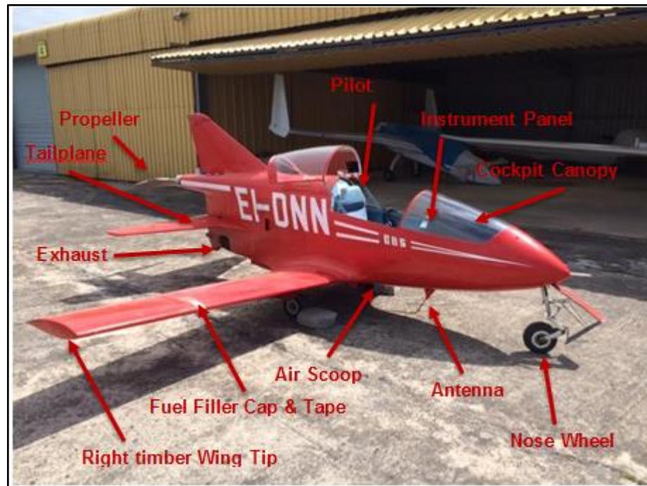
Photo No. 1: annotated photograph of the accident aircraft
