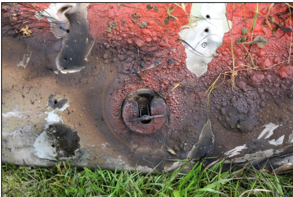
Photo No. 7: Left-hand wing fuel cap (as found)
