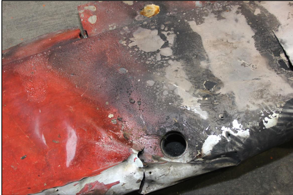
Photo No. 8: Right-hand wing without fuel cap (as found)
