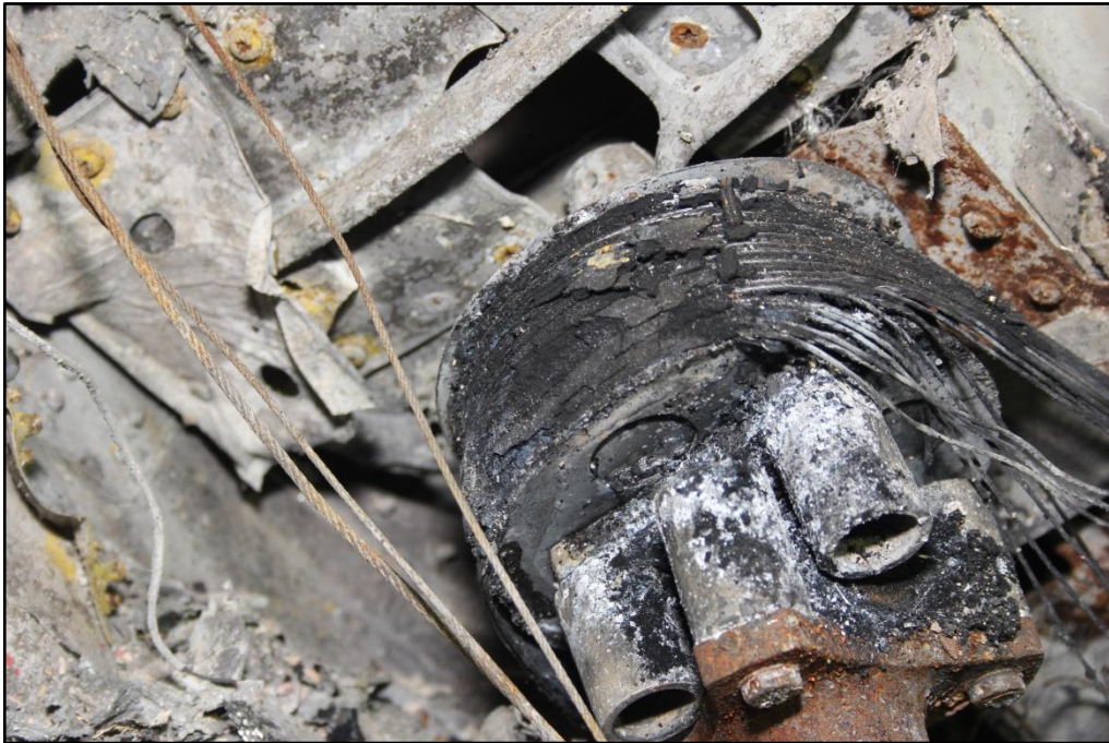
Photo No. 6: Fire-damaged Propeller Drive belt
