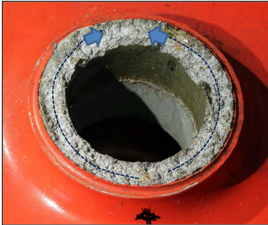
Photo No. 9: Fractured propeller attachment spigot
