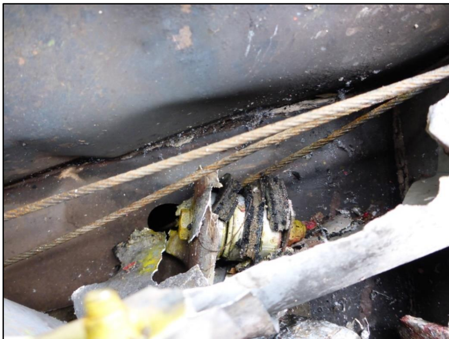
Photo No. 5: Damaged elevator pulley block
